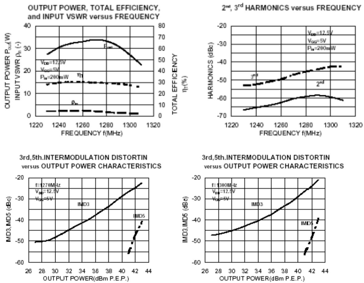
**ELECTRICAL CHARACTERISTICS** ( $T_{case}=+25^{\circ}\text{C}$ ,  $Z_G=Z_L=50\Omega$ , unless otherwise specified)
