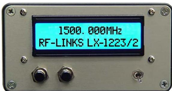
The new Audio/Video transmitter is a special design for Military applications capable to work in extremely low or high temperature range. This transmitter has wide range of frequencies from 1200 MHz- 2300 MHz with no gaps or limits. This transmitter has digital display. It is easy to change channels using 2 push buttons Up / Down. This transmitter has 2 W RF power thank to special wideband circuitry. LX-1223/2 works from 9 V- 16 V.
